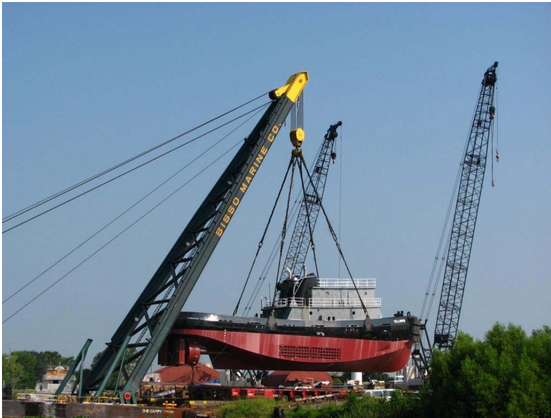
Bisso Marine uses the D/B CAPPY BISSE to launch the M/V YELLOWFIN.
