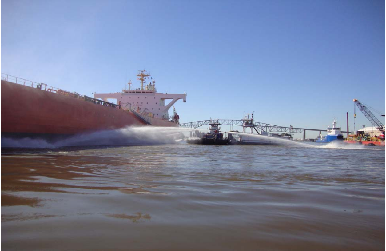
T&T MARINE uses 3,300-gpm fire pumps to decontaminate the oil tanker's hull following the collision.
