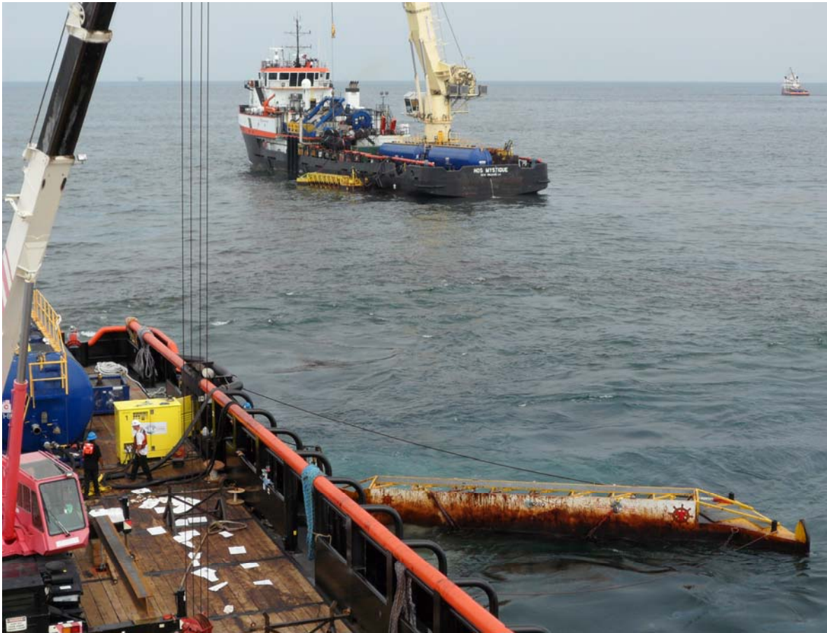
Two OSV's outfitted with T&T MARINE skimming systems operate in the Gulf of Mexico.
